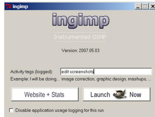
**Figure 2.** The ingimp start-up screen allows users to describe their intended task, visit the website to view personal statistics, or launch GIMP. Users also have the option of disabling logging each time the application is started.
