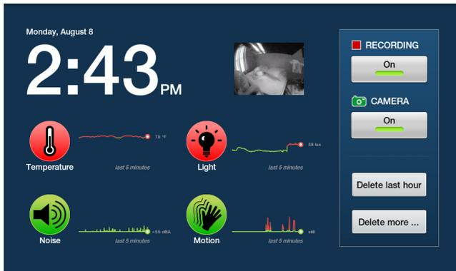
**Figure 3. The home screen, with clock, current sensor state, and controls. Each sensor has a sparkline of recent readings, colored red if those readings are outside recommended thresholds for a good sleep environment.**
