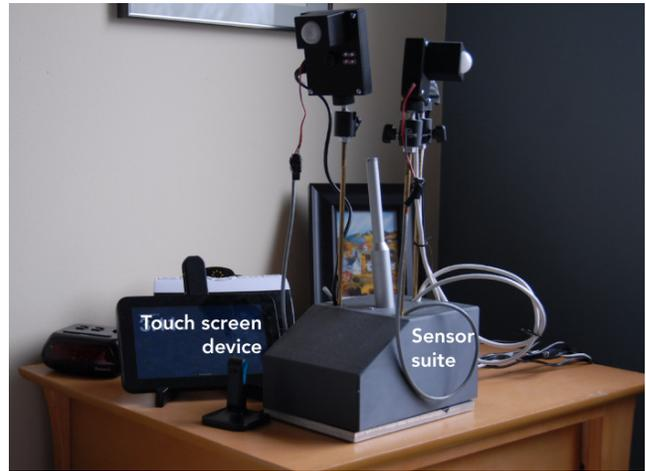
**Figure 2.** Lullaby deployed on bedside table. Visible here are the touchscreen tablet mounted in a stand for easy access from the bed and the sensor box with pivoting sensor enclosures. The sensor suite itself is about the size of a bedside lamp.
